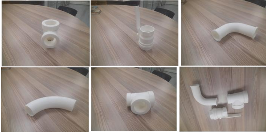
Figure 2: Some of the 3D printed substructures.
