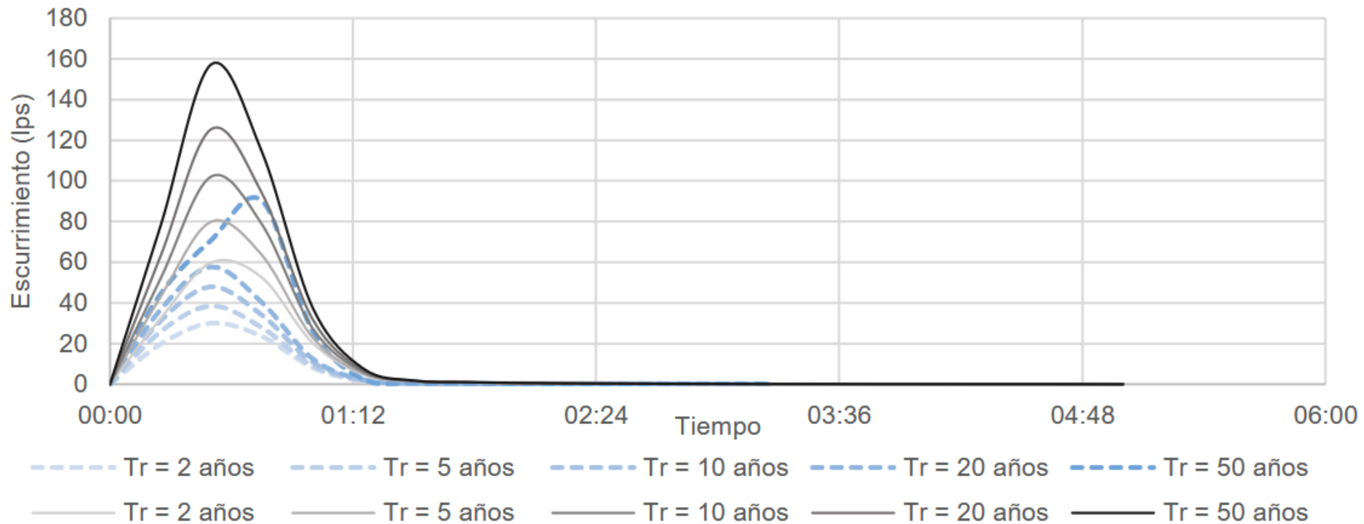
Runoff Hydrographs: Natural condition (solid lines) vs. Technique IV (dotted lines) for a 60-minute storm and various return periods.
