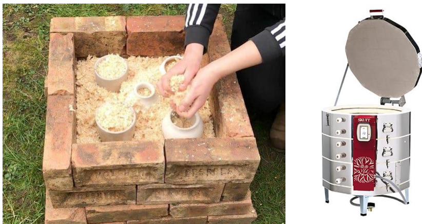
Figure 09: Left: Self-built sawdust brick kiln. Right: Modern electric SKUTT kiln.
